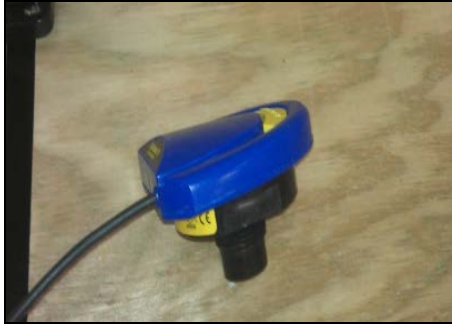
Figure 43: Tank level meter
